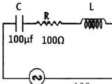
$$V_{max} = 100V, f = \frac{100}{\pi} \text{ Hz}$$
